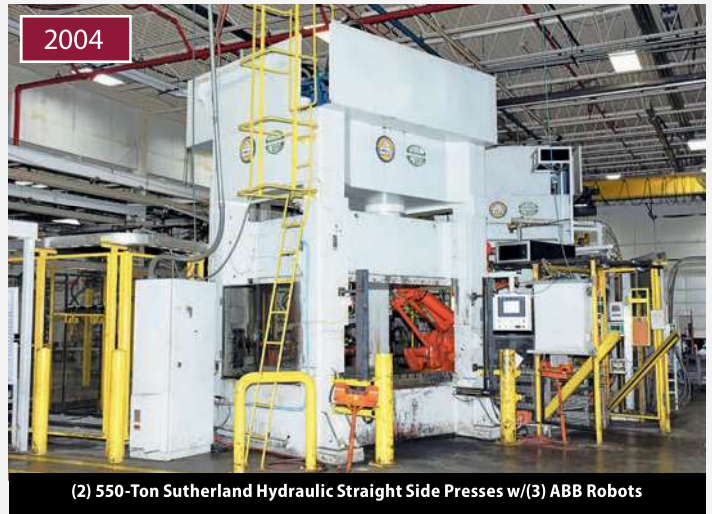
Tandem Hydraulic Press Line: (5) Sutherland Hydraulic Presses w/Quick Die Change and ABB Robots
