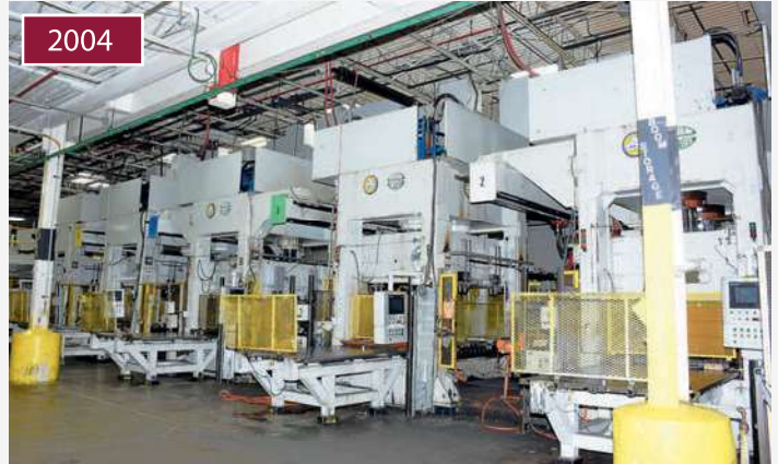
Tandem Hydraulic Press Line: (5) Sutherland Hydraulic Presses w/Quick Die Change and ABB Robots
