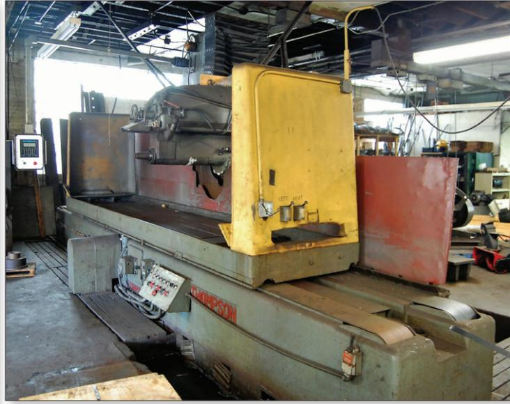
**ROTARY SURFACE GRINDER:** 84" Blanchard with 150 HP Motor;
