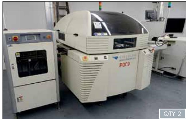
MPM Speedline UltraFlex 3000 Stencil Screen Printer
