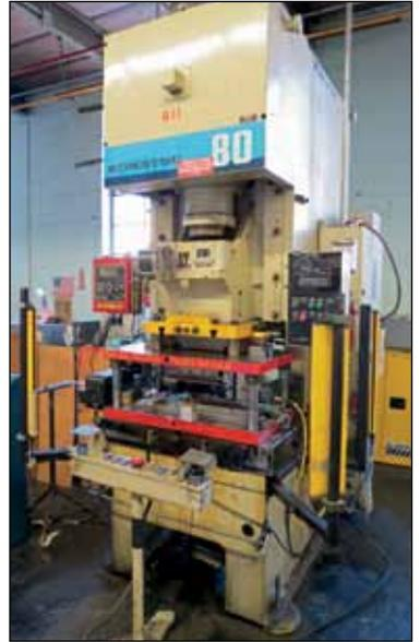
Komatsu OBS-80-VS-3 Gap Frame, 88 Ton, 37 - 75 SPM
