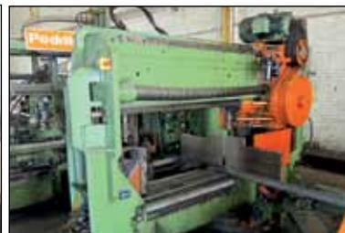
Peddinghaus Beam Drill & Saw Line, Model TDK 10009G Drill
