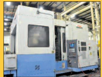
Mazak HV800 CNC HMC
