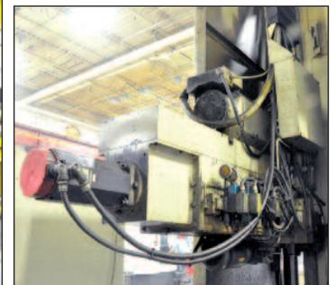
• OLYMPIA HT 120 X 80 CNC TABLE TYPE HORIZONTAL BORING MILL, GE FANUC 16i-M CNC, X-118"; Y-63"; Z-28"; W-39"; 49" x 63" B-Axis Rotary Table, 360,000 Positions, 22,000 Lbs. Table Cap. 6-3000 RPM, Thru Spindle Coolant, 2000, S/N 337-0E00
