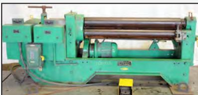
**STE-CO** IP 2 initial pinch bending rolls
