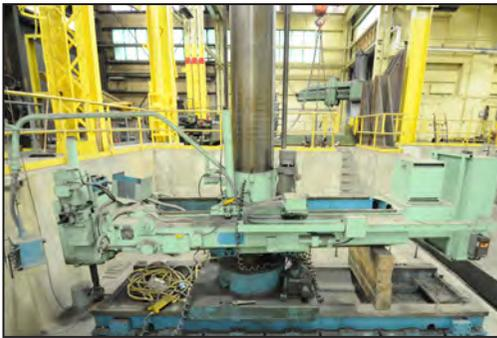
**GIDDING & LEWIS 140 U CNC portable universal drilling, tapping and boring machine**
