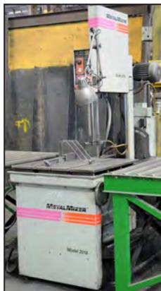
**METALMIZER vertical band saw**
