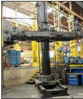
**KAUKAUNA portable universal drilling, tapping & boring machine**
