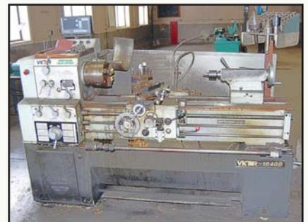
16" x 40" Victor 1640B Gap Bed Lathe
