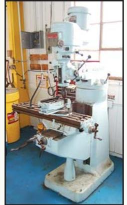
Bridgeport "Series I" 2HP Vari-Speed Vertical Mill
