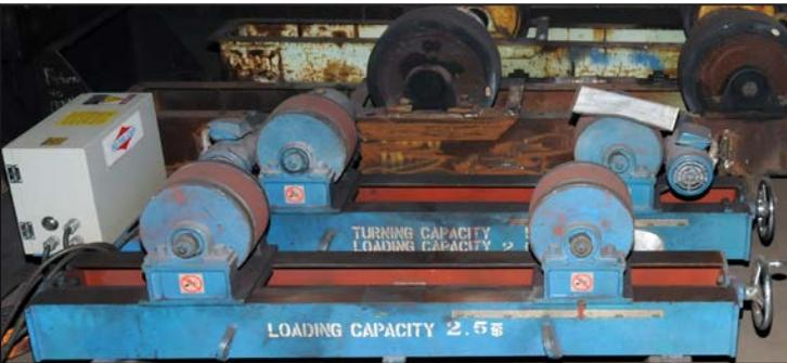
Partial view of tank turning rolls available
