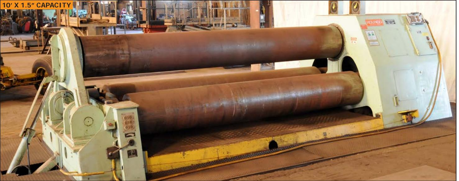
ROUND O PS 460/10 hydraulic double pinch plate bending rolls
