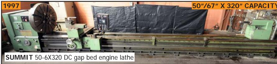
SUMMIT 50-6X320 DC gap bed engine lathe
