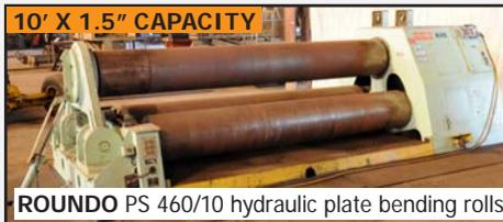
ROUND0 PS 460/10 hydraulic plate bending rolls
