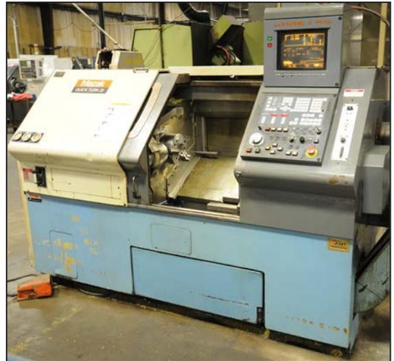
MAZAK QT 20 CNC turning center
