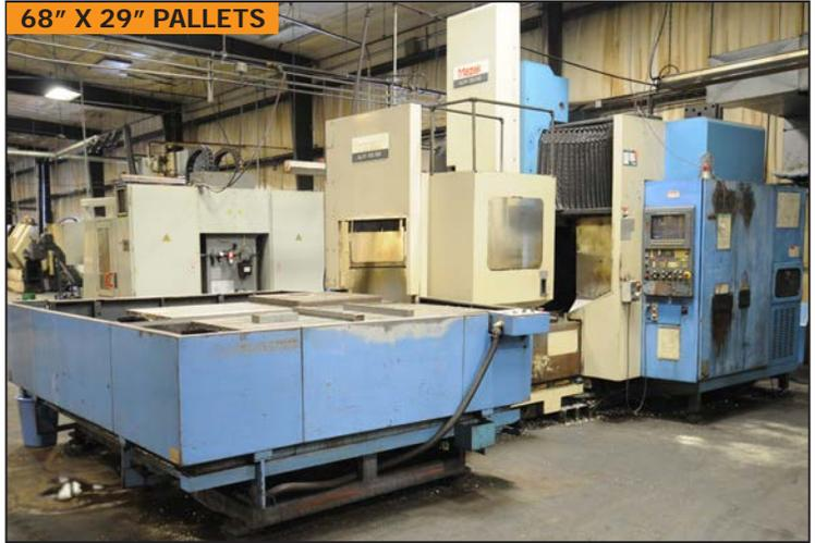
MAZAK AJV-35/60 twin pallet CNC vertical machining center
