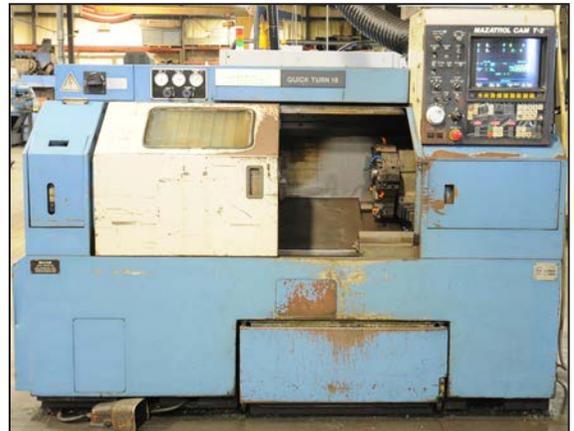
MAZAK QT 15 CNC turning center
