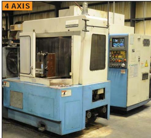
MAZAK H-400/40 twin pallet CNC horizontal machining center
