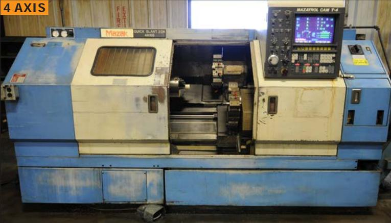
MAZAK QT 20N twin turret CNC turning center
