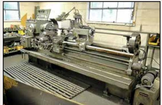
Lodge & Shipley AVS Mdl. 2013 20" x 78" Geared Head Engine Lathe
