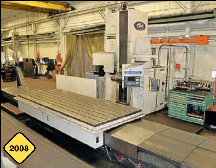
Toshiba Mdl. BP-150.P45 CNC Table-Type Horizontal Boring Mill
