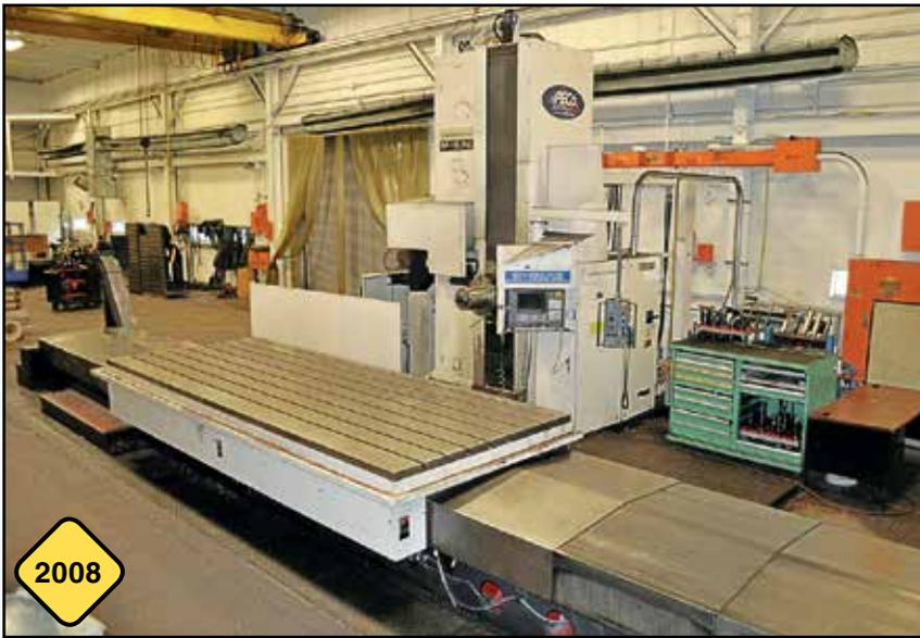
Toshiba Mdl. BP-150.P45 CNC Table-Type Horizontal Boring Mill
